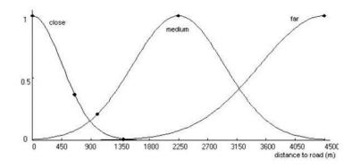
**Figure 3.37** A case of fuzzy membership function according to the distance to the road when defining new locations for industrial sites (Source: Yanar, T.,A., Akyurek, Z. 2004. The enhancement of ArcGIS with fuzzy set theory. ESRI International User Conference, 30. June 2004: 16 str. http://proceedings. esri.com /library/userconf/proc04, 15.12.2010)
